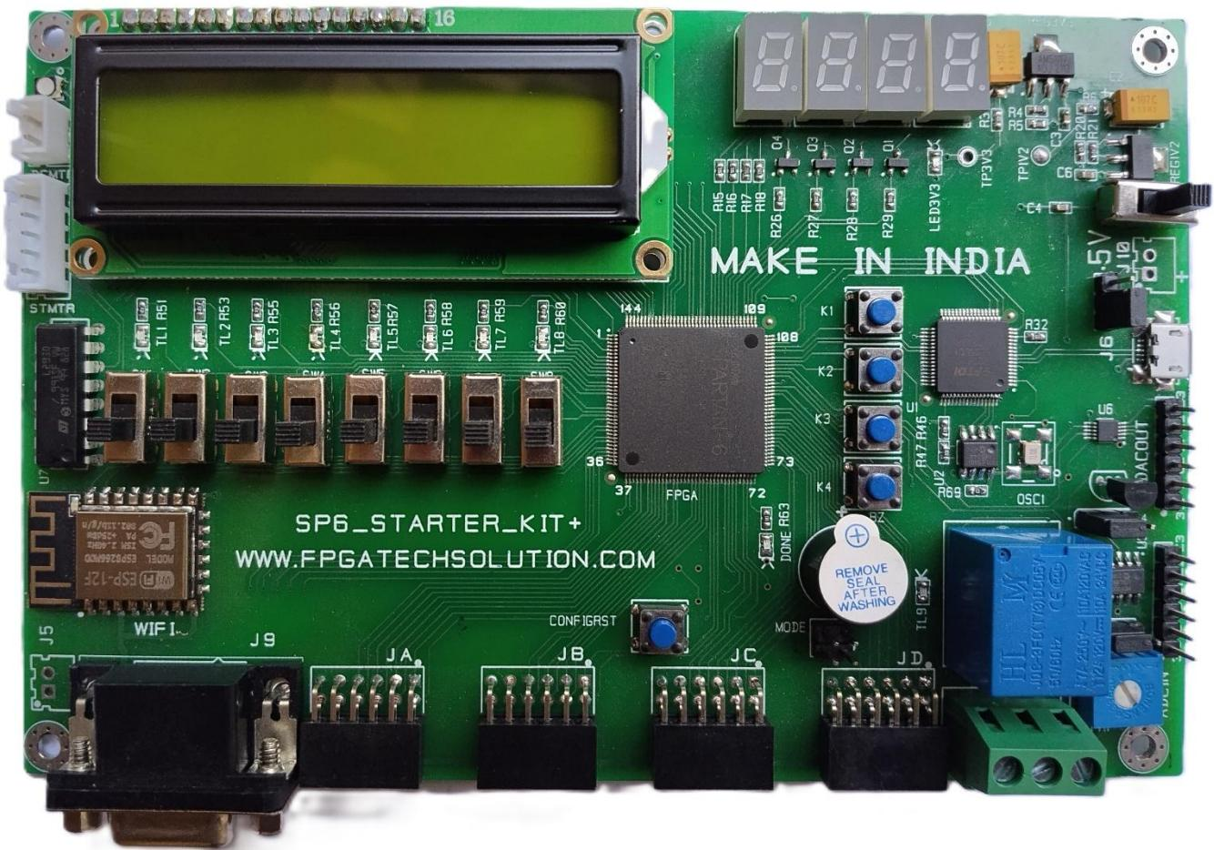
The Spartan6 starter kit is a complete, ready-to-use digital circuit development platform based on the latest Spartan6 Field Programmable Gate Array (FPGA) from Xilinx. With its high-capacity FPGA, low overall cost, and collection of USB, VGA and other ports, the Spartan6 starter kit can host designs ranging from introductory combinational circuits to complex sequential circuits like embedded processors and controllers.
